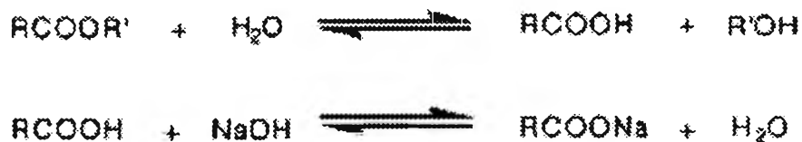
Figure 2.6 Saponification of fatty acid alkyl ester.
