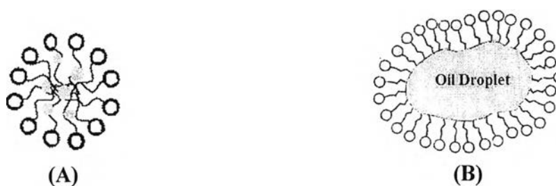
Figure 2.20 A) solubilization and B) emulsification.
