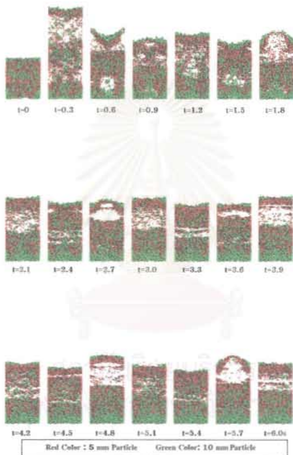
Figure 45. Solids movements at the axially sliced two-dimensional center region, superficial gas velocity = 3.5 m/s, particle size 10mm/5mm ( d_p/d_s = 2.0 )
