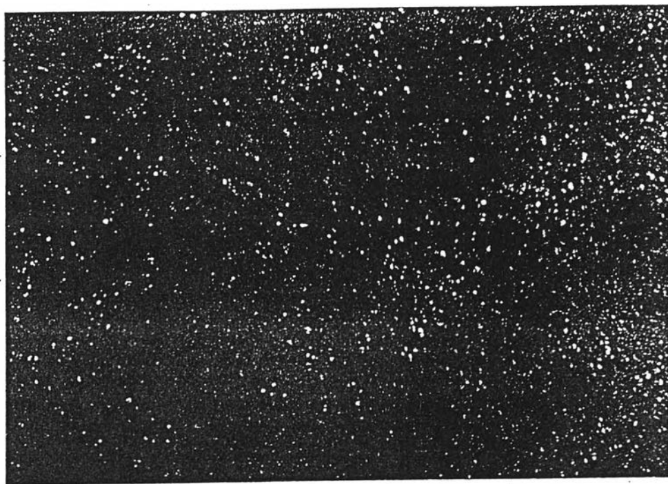
Figure C-1 PVC/PPY from 25%FeCl 3 , 25%pyrrole, at-15°C and 20 hrs. for polymerization.
