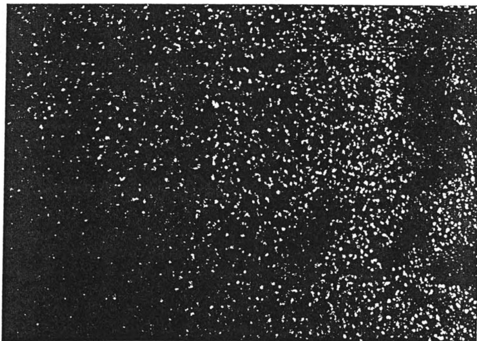
Figure C-6 LDPE/PPY from 25%FeCl 3 , 25%pyrrole, at 30°C and 20 hrs. for polymerization.
