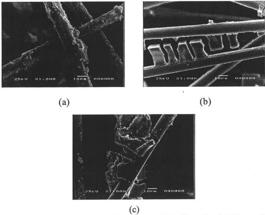
Figure 4.2 SEM micrographs of (a) Degussa P25, (b) sol-gel TiO<sub>2</sub>, and (c) 1%Pt/sol-gel TiO<sub>2</sub> coated on glass wool.
