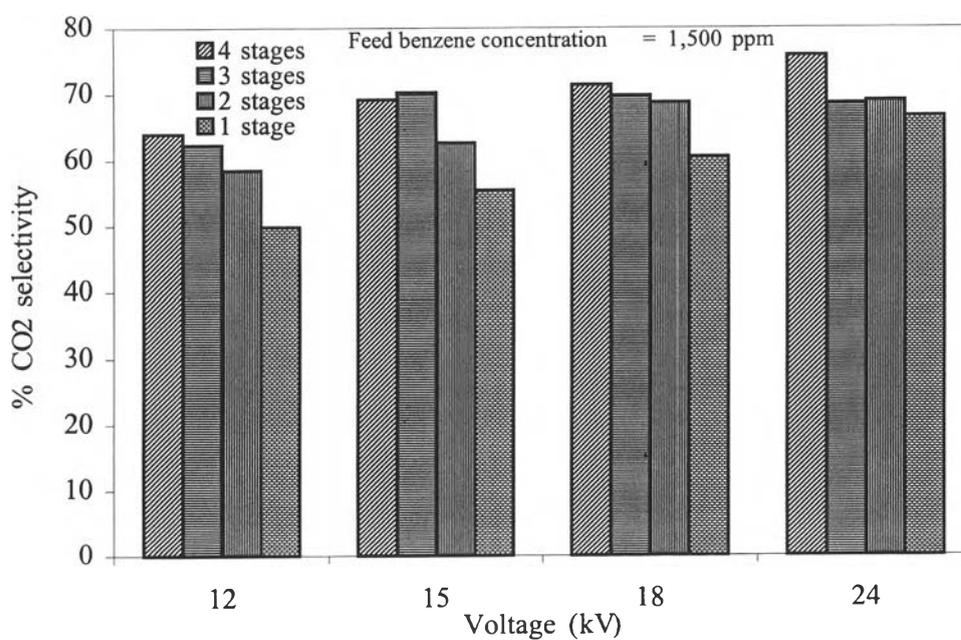
**Figure 4.11** Effect of applied voltage on CO<sub>2</sub> selectivity at different stage number of reactors at feed flow rate of 500 ml/min, 300 Hz, and a gap distance of 1 cm.
