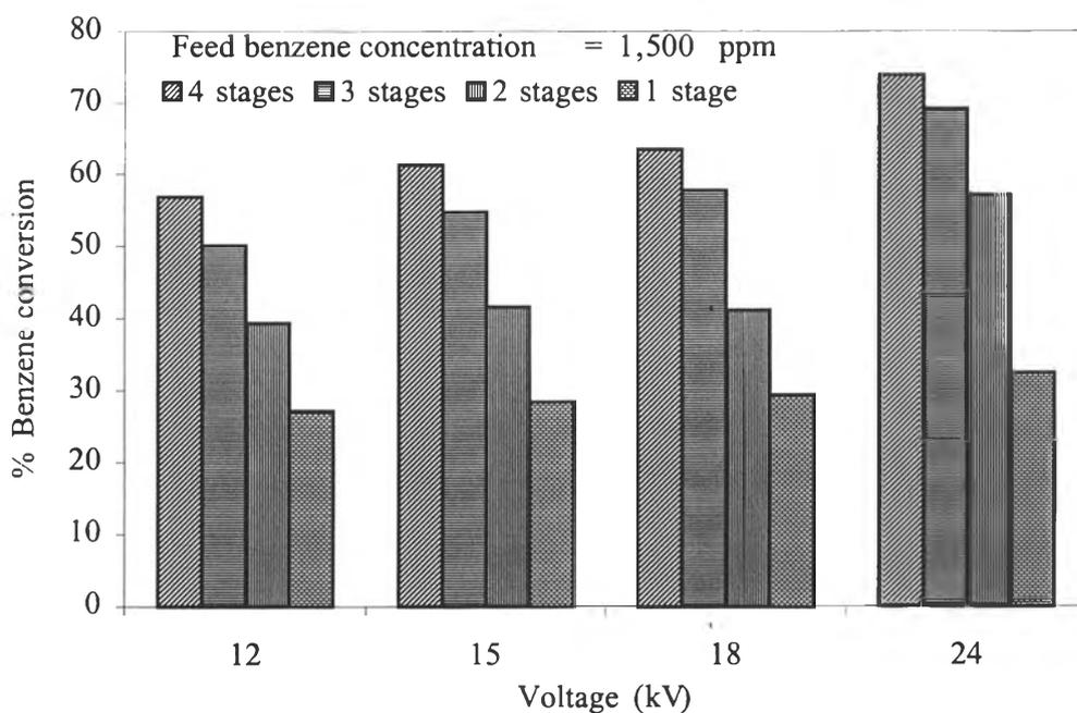
**Figure 4.8** Effect of applied voltage on benzene conversion at different stage number of reactors at a feed flow rate of 500 ml/min, 300 Hz, and a gap distance of 1 cm.
