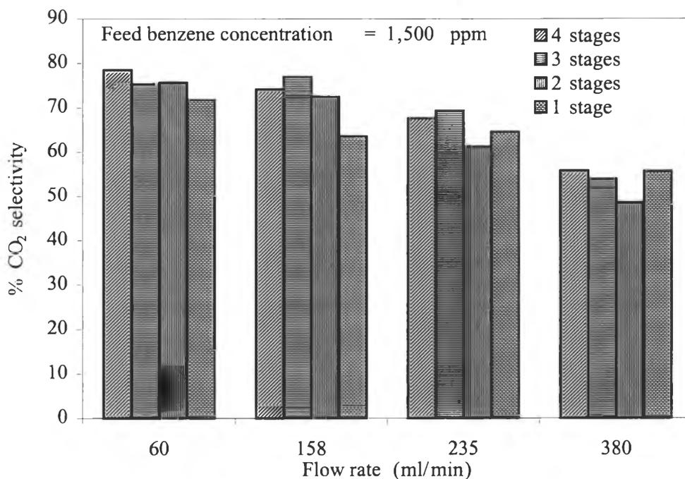
**Figure 4.14** Effect of feed flow rate on CO<sub>2</sub> selectivity at different stage number of reactors at 15 kV, 500 Hz, and a gap distance of 1 cm.
