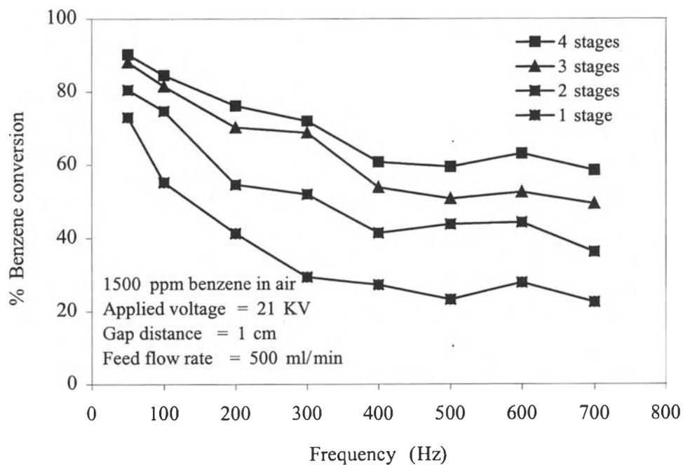
**Figure 4.3** Effect of frequency on benzene conversion at different stage number of reactors at 21 kV.
