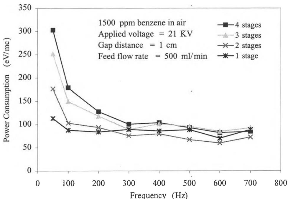
**Figure 4.7** Effect of frequency on power consumption of benzene at different stage number of reactors at 21 kV.
