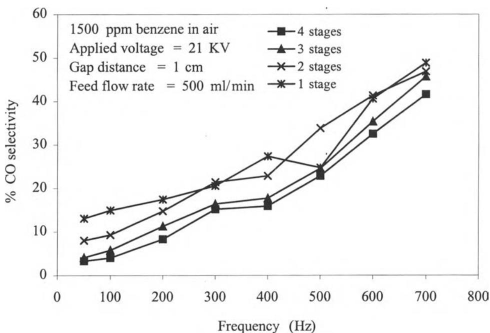
**Figure 4.5** Effect of frequency on CO selectivity at different stage number of reactors at 21 kV.
