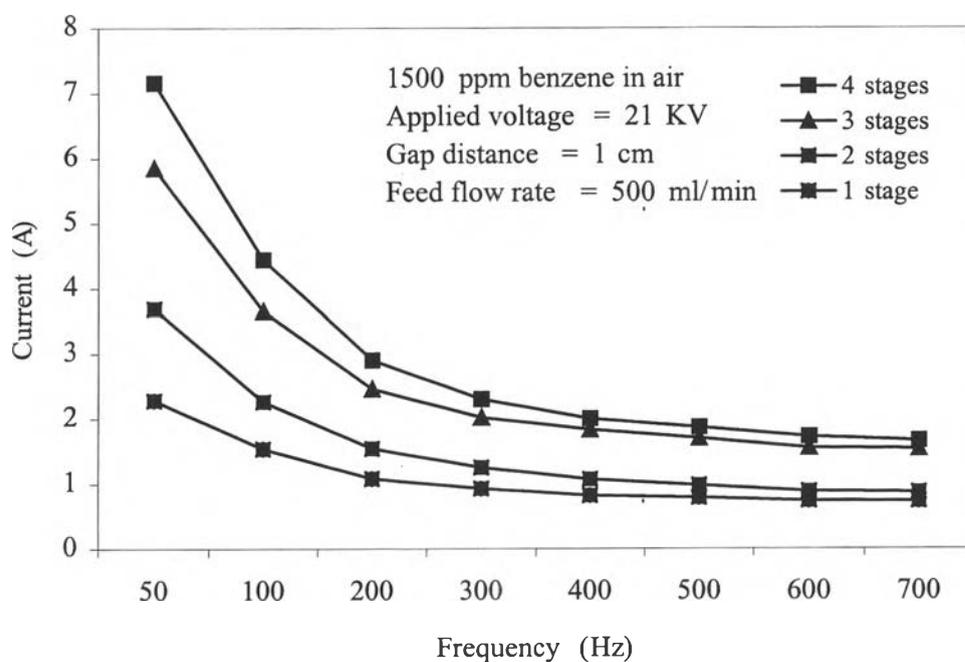
**Figure 4.4** Effect of frequency on current at different stage number of reactor at 21 kV.
