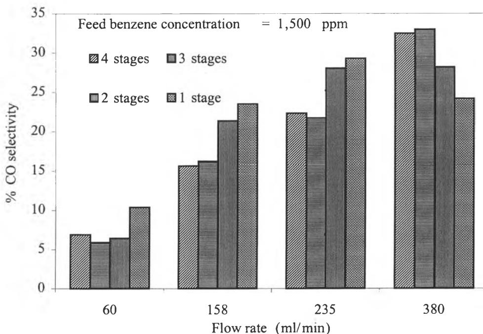
**Figure 4.13** Effect of feed flow rate on CO selectivity at different stage number of reactors at 15 kV, 500 Hz, and a gap distance of 1 cm.
