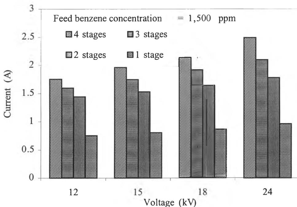
**Figure 4.9** Effect of applied voltage on current at different stage number of reactors at a feed flow rate of 500 ml/min, 300 Hz, and a gap distance of 1 cm.
