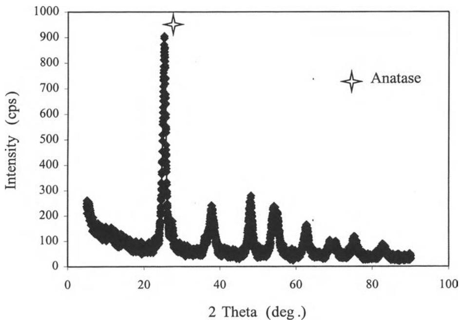
**Figure 4.1 (b)** XRD pattern of sol-gel  $TiO_2$ .
