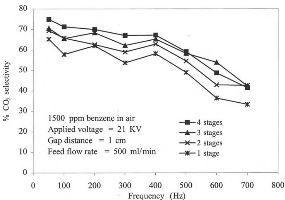
**Figure 4.6** Effect of frequency on CO<sub>2</sub> selectivity at different stage number of reactors at 21 kV.
