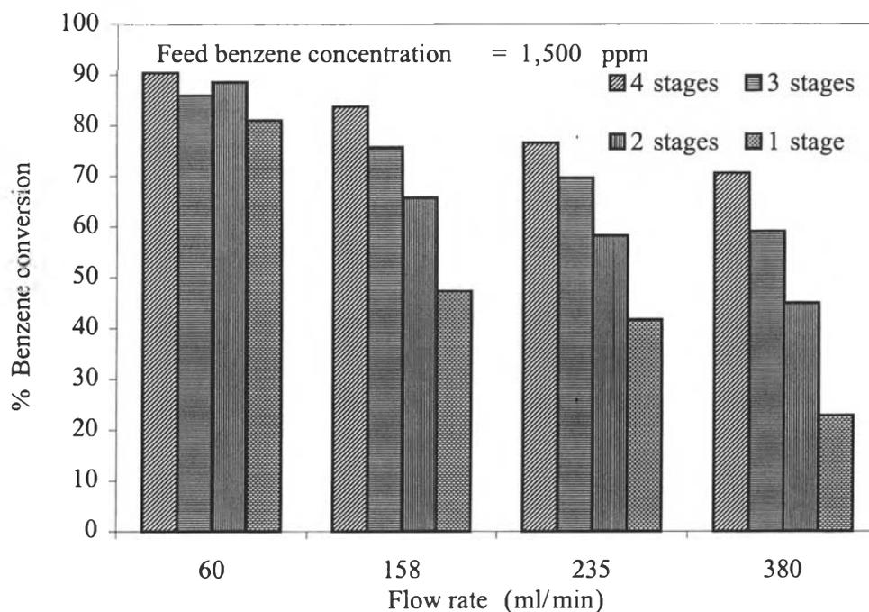
**Figure 4.12** Effect of feed flow rate on benzene conversion at different stage number of reactors at 15 kV, 500 Hz, and a gap- distance of 1 cm.
