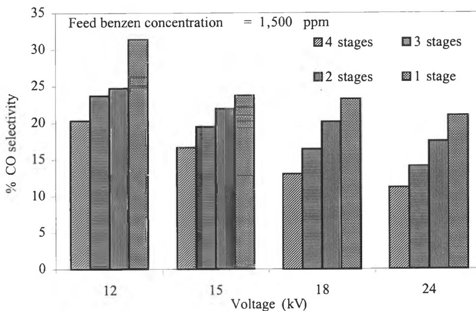
**Figure 4.10** Effect of applied voltage on CO selectivity at different stage number of reactors at feed flow rate of 500 ml/min, 300 Hz, and a gap distance of 1 cm.
