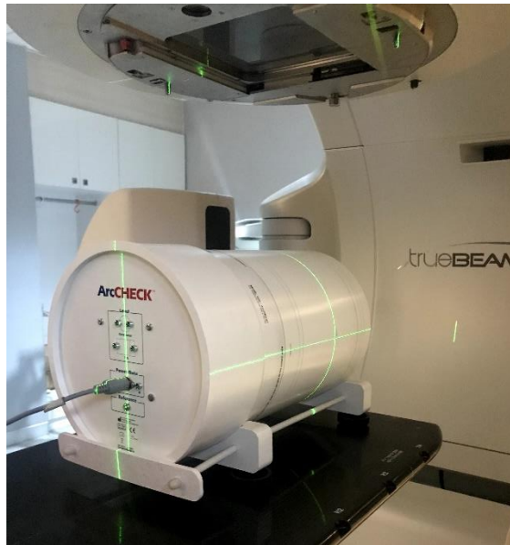
Figure 3. 4 The setup of ArcCHECK phantom
