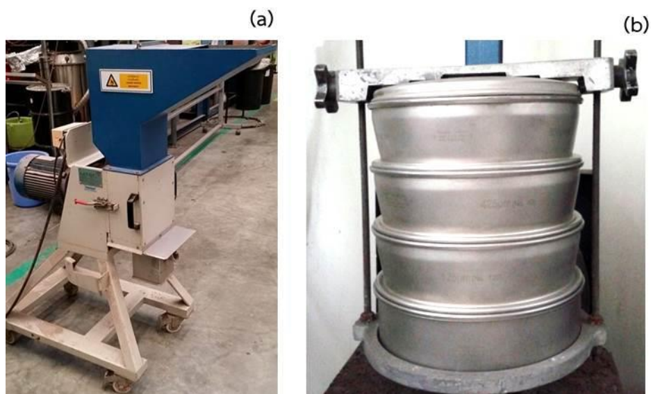
Fig. 3.2 Instruments for preparation the Jatropha residues (a) Grinding machine (b) Sieve shaker
