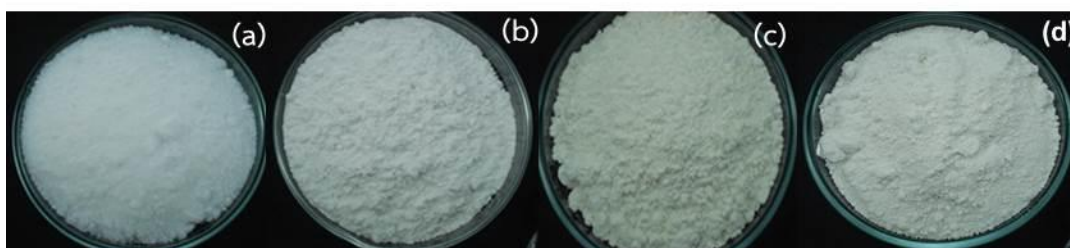
Fig. 3. 6 Physical appearances of support catalysts (a) alumina ( \text{Al}_2\text{O}_3 ) (b) \text{ZrO}_2 (c) rutile based ( \text{TiO}_2 ) and (d) anatase ( \text{TiO}_2 )
