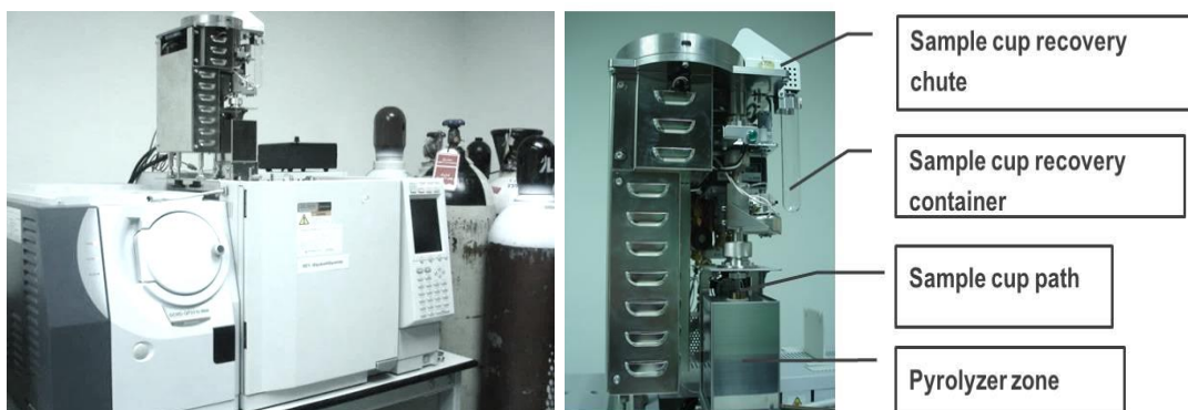
Fig. 3. 18 A pyroprobe (multifunctional pyrolyzer, PY-2020iD, Frontier Lab) interfaced to a gas chromatograph coupled to a mass selective detector (GCMS- QP2010, Shimadzu)
