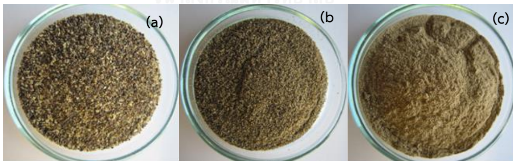
Fig. 4.1 Jatropha residues obtained from Chiangrai province after size reduction; (a) 0.425-0.85 mm (b) 0.125-0.425 mm (c) < 0.125 mm
