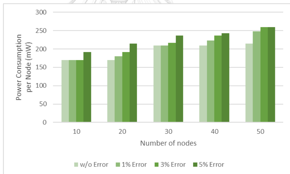
Figure 21 Graph showing comparison of average power consumption per node in the disseminations using our algorithm with multiple rates of intermittent faults as number of nodes increasing
