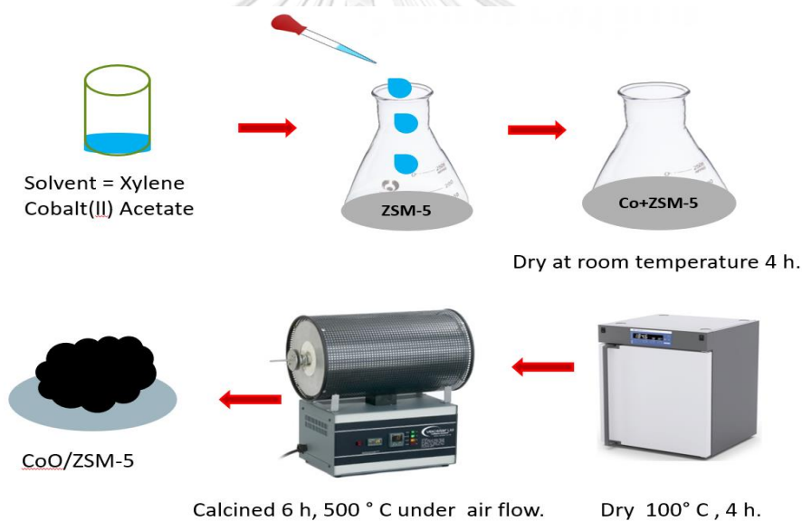
Figure 3 Catalyst preparation by incipient wetness impregnation method
