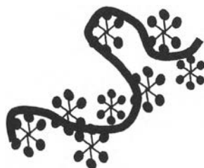
Figure 5.2 The proposed model for PEO-HTAC complex in 0.1 M \text{KNO}_3 solution at maximum binding.
