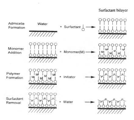
Figure 1.1 The four-step admicellar polymerization process.
