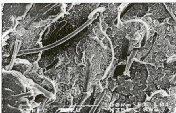
Figure 4.16 SEM micrographs of the impact fracture surface of MMA-g-HDPE/silk by one-step reactive blending method with (A) 10%, (B) 20%, (C) 30% silk contents.
