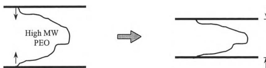
Figure 4.23 Schematic illustration of bridging flocculation occurs in polymer nanocomposite in the presence of high molecular weight polymer.
