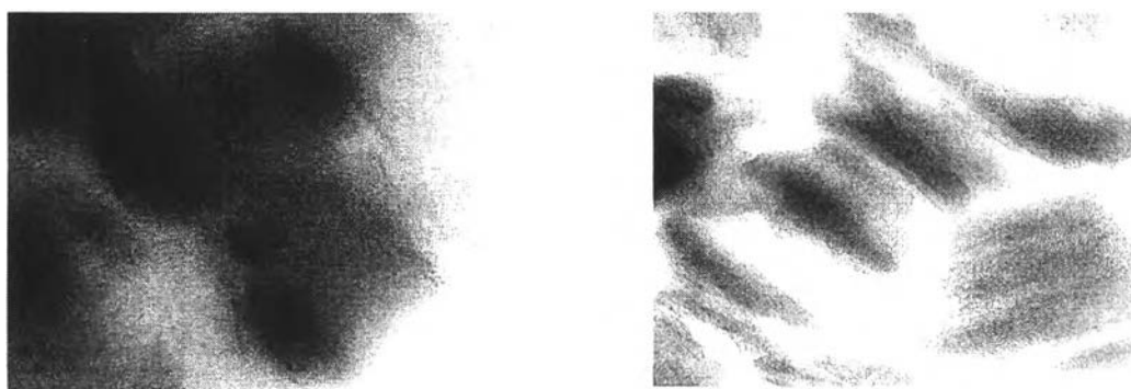
Figure 4.6 Transmission electron micrographs of (a) TA-clay catalyst at 150,000X magnification, and (b) Mo-V-clay catalyst at 150,000X magnification.
