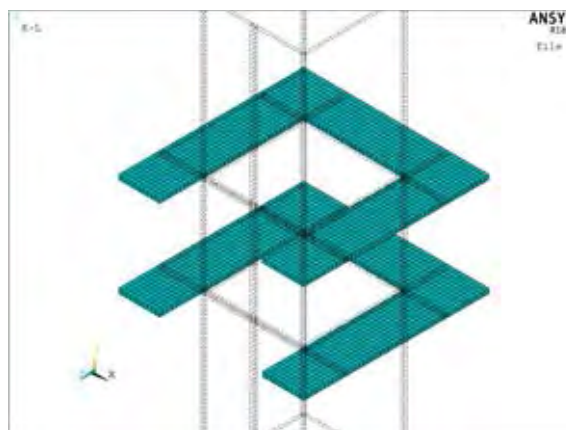
Figure 3.6 Geometry of external ring stiffener
