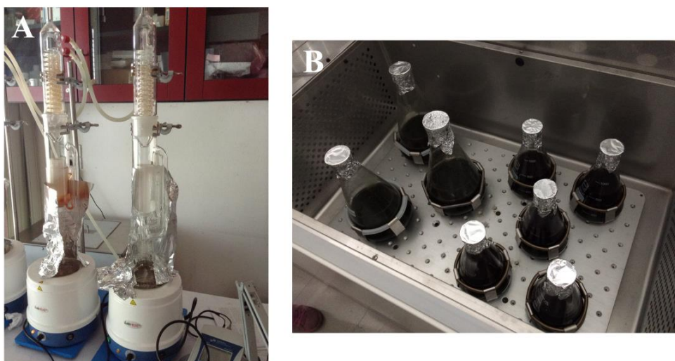
Figure 17: Plant extract preparation using (A) Soxhlet apparatus and by (B) maceration in a shaking incubator
