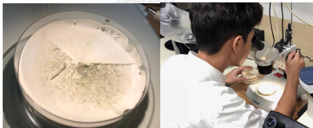
Figure 10 Filtered cellulose nitrate membrane in a closed dish and the screening for microplastics by a stereomicroscope.
