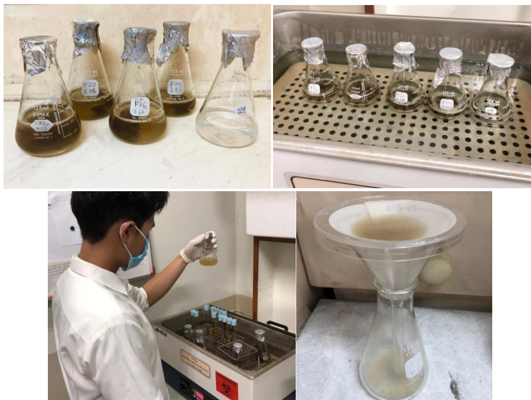
Figure 9 Digestion of tissue sample in glass flasks, incubation and filtration.
