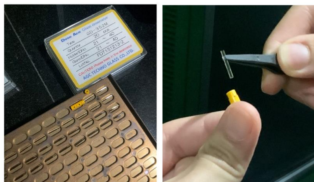
Figure 3.11 Radiophotoluminescent glass dosimeter (RPLGD).
