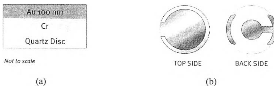
Figure 3.2 The structures of (a) gold layer and (b) sensor layout of gold crystal.
