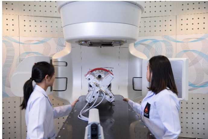
Figure 33 Delta4 phantom setup for measurement
