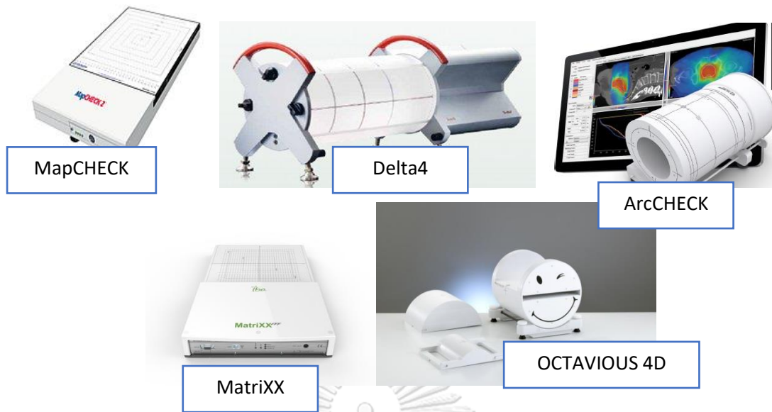
Figure 2.13 Commercial products of measurement-based with phantom devices for patient-specific QA
