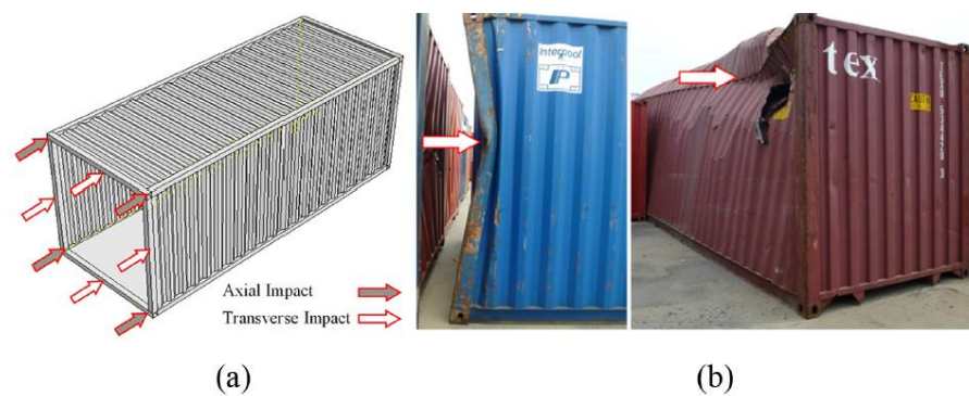
Figure 2.16 (a) Axial and transverse impact configurations for a shipping container and (b) damaged shipping containers under the transverse impact [20]
