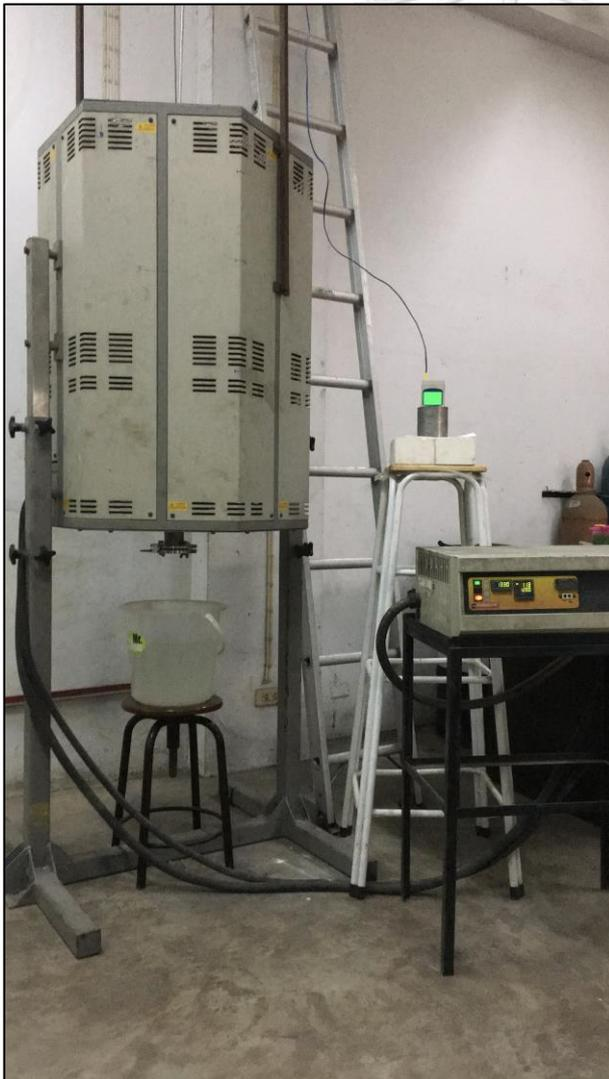
Figure 3-3 Establishment of vertical tube furnace
