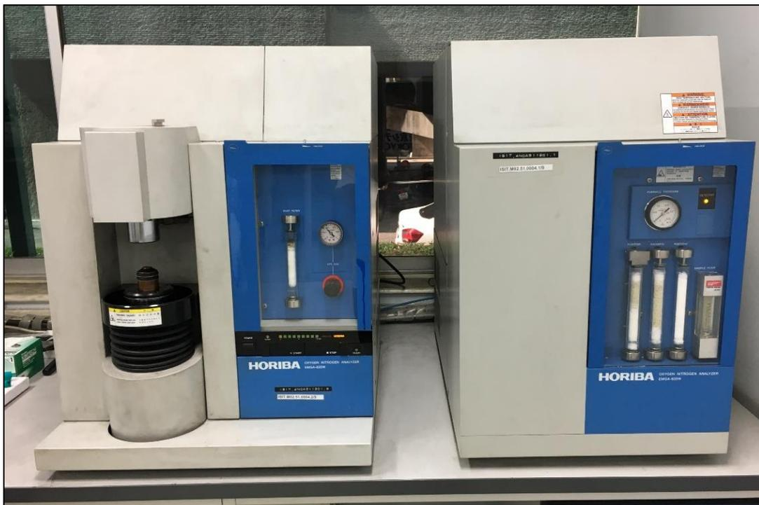
Figure 3-5 Optical emission spectroscopy (Spectrolab LAVM12) (left) and oxygen/nitrogen analyzer (EMGA-620W) (right)
