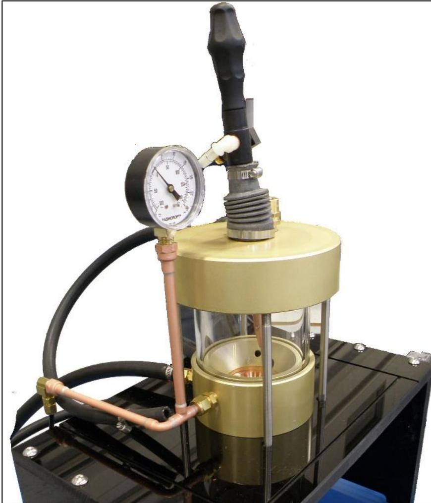
Figure 3-1 Vacuum single arc melting furnace (model SA-200 MRF) with pressure guage
