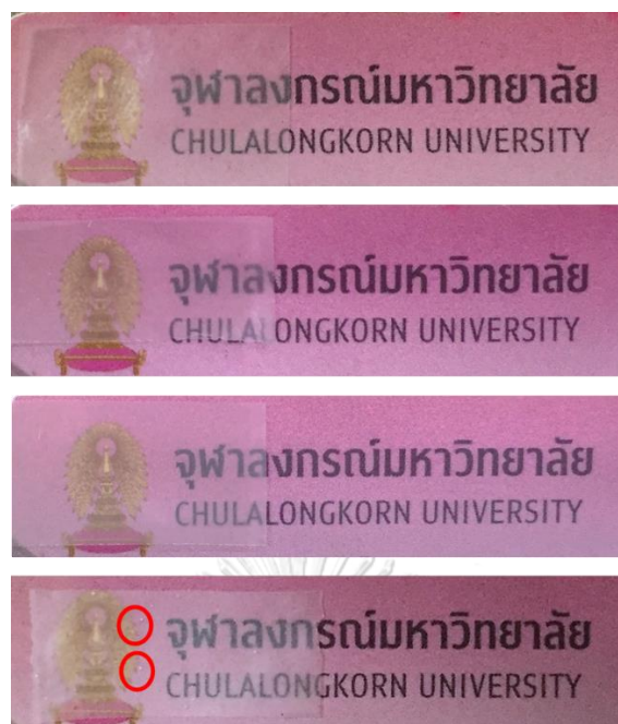
Figure 5.14 images of pure cellulose nanopaper (A) and cellulose nanopaper filled with ZnO nanoparticles at contents of 1 wt% (B), 3 wt% (C), and 5 wt% (D).
