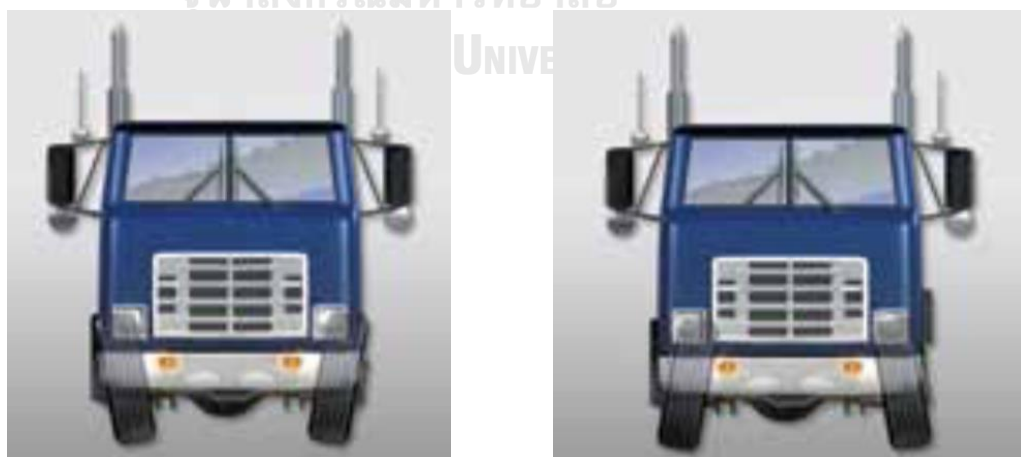
Figure A.10 Positive camber (left) and negative camber (right) in front of view
