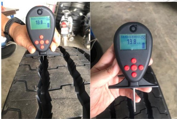
Figure 4.7 Placing the probe and measuring all circumferential grooves
