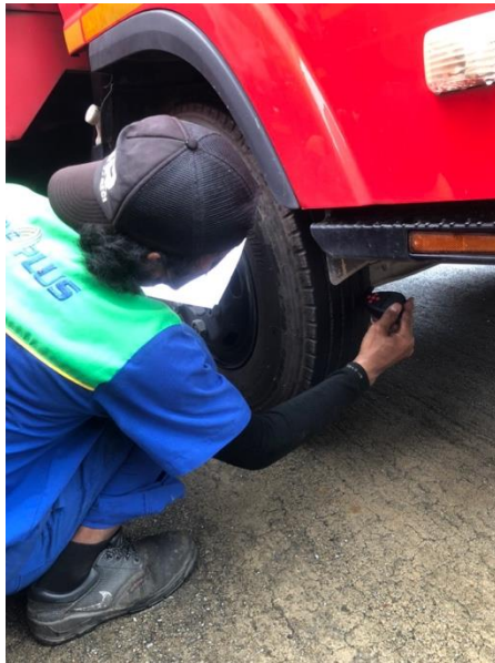
Figure D.1 Tread depth measurement
