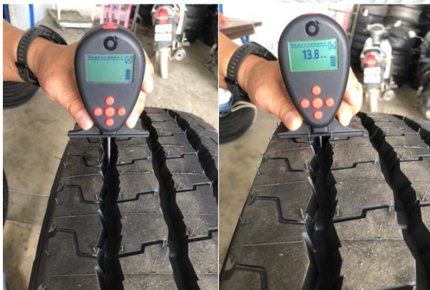
Figure 4.4 Placing a probe for measurement
