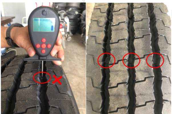
Figure 4.5 Avoiding tread wear indicators
