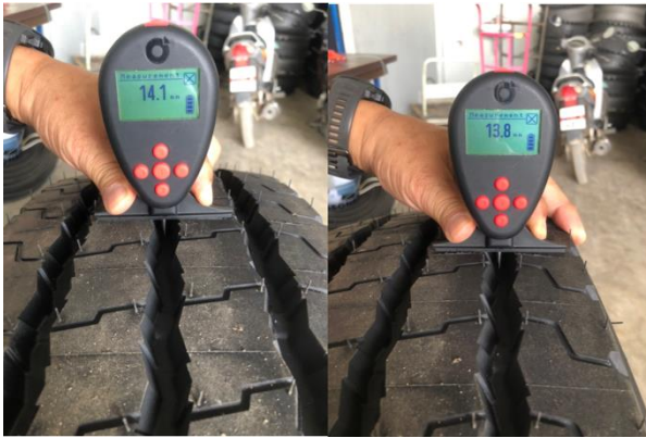
Figure 4.6 Reading tread depth
