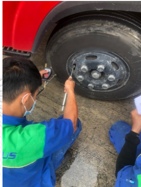
Figure D.2 Air pressure measurement
