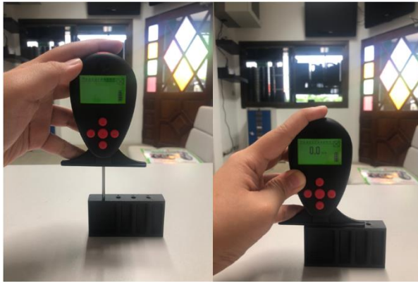
Figure 4.3 Setting zero for tread depth gauge
