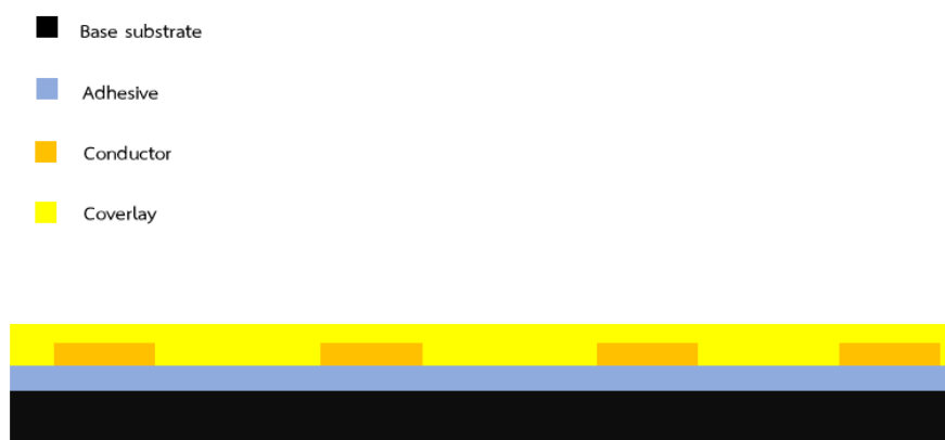
Figure 2.1 Flexible printed circuit board make up
