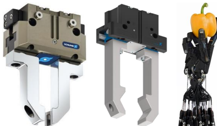
Figure 7 Parallel jaw gripper (left)[10], specialized jaw gripper (middle)[11], and robot hand (right)[12]
