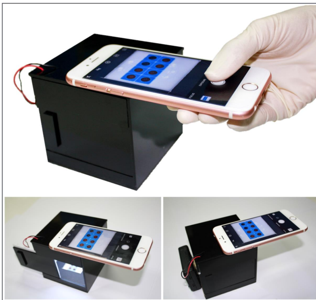
Figure 3.1.1 Photograph showing the setup of an in-house light control box with the smart-phone for \text{Cl}^- detection.
