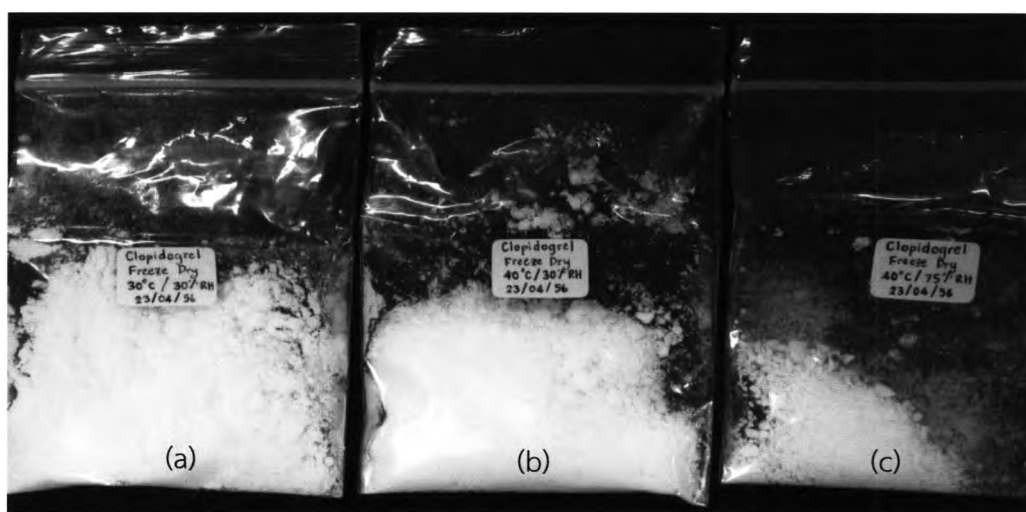
Figure 73 Polyamorphous samples obtained by freeze drying method and stored for 7 days at 30°C 30%RH (a) 40°C 30%RH (b) and 40°C 75%RH (c)
