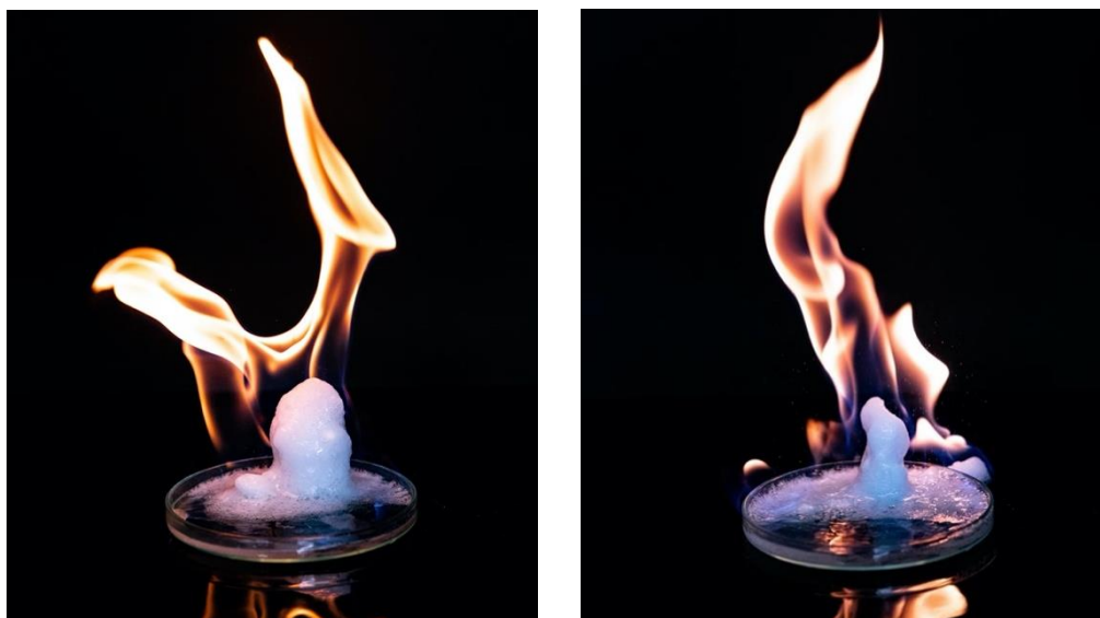
Figure 2.3 Methane hydrate pellet samples (Pictures taken in The Petroleum and Petrochemical College, Chulalongkorn University, Bangkok, Thailand).
