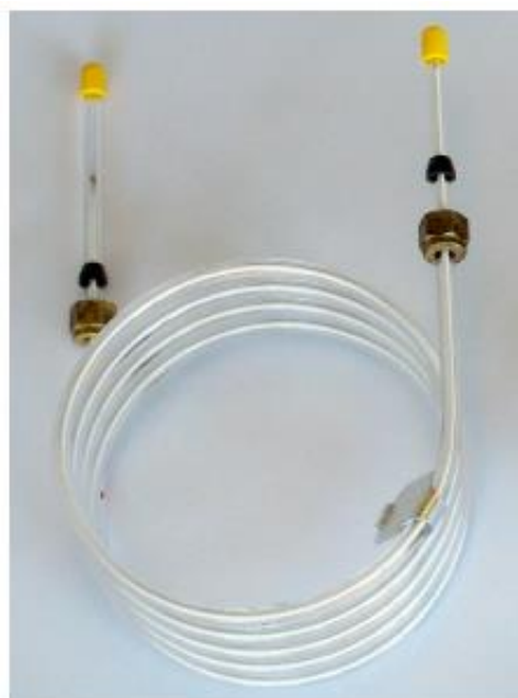
Figure 2.14 Packed column of gas chromatography (Piantanida and Barron, 2014).
