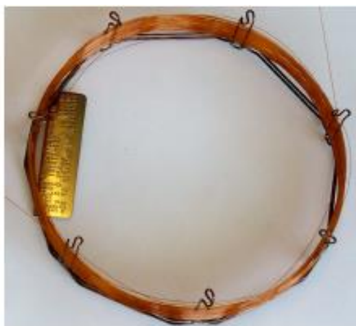
Figure 2.13 Capillary column of gas chromatography (Piantanida and Barron, 2014).
