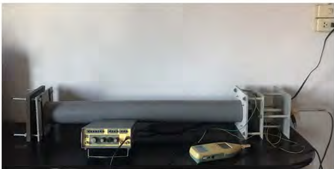
Figure 3.5 Measurement setup for the sound absorption test.
