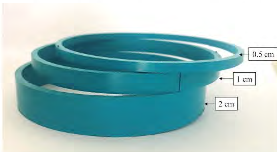
Figure 3.2 PVC mold 10.5cm diameter (thickness: 0.5cm, 1cm, and 2cm).
