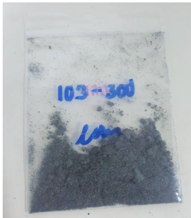
Figure A.4 MPs particles after immersed in wastewater from sugar factories
