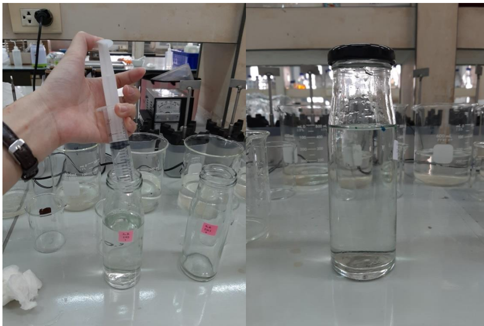
Figure A.6 Collection of suspension for MPs analysis with stereo microscope
