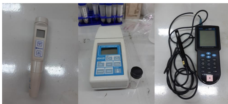
Figure 3.3 Laboratory instruments for measured (A) pH, (B) turbidity, and (C) conductivity.
