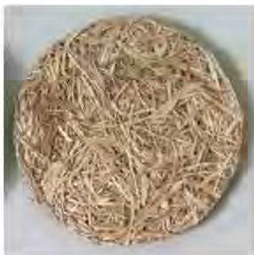
Figure 4.1 The acoustic absorption board from banana pseudo-stem
