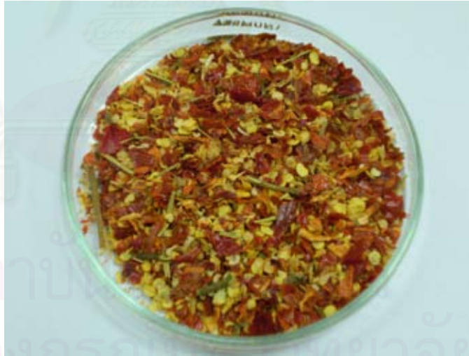
Figure 4.3 Dried ground chili pepper passing 13 mm opening of Hammer mill
