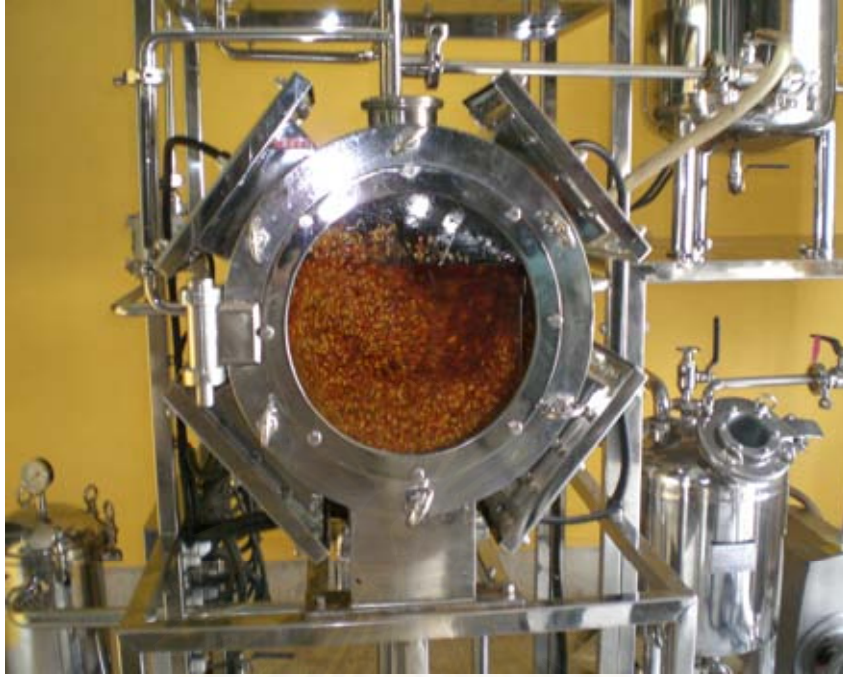
Figure 4.4 The pilot scale 20-L ultrasonic extractor
