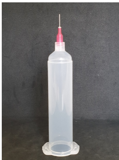
Figure 2.1 3D-printing syringe with 25-gauge blunt needle.
