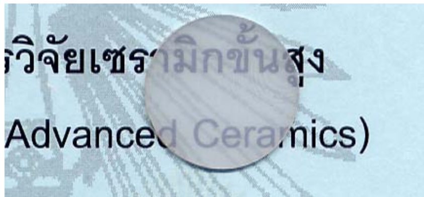
Fig. 4.17 Transparency of conventional sintered \text{Al}_2\text{O}_3 specimen (CV-5)
