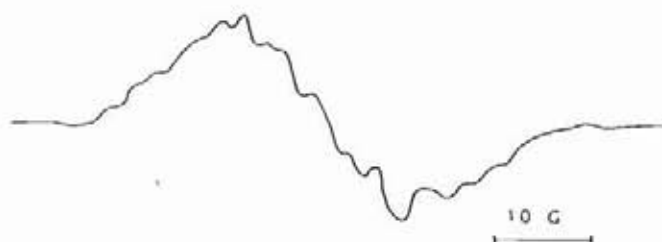
Fig. 5. ESR spectrum of 1-chlorobutadiene-DCA adduct, \gamma -ray irradiated at -78^{\circ}\text{C} and measured at room temperature.
