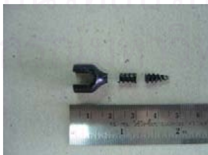
Fig. 9B Photograph of the specimens after autoclaving in H_2O_2 and incubating in R-SBF solution
