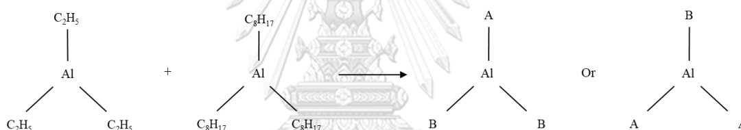
Scheme 4. 1 The possible new alkyl aluminum to produce suitable activators (A and B refer to randomly -C 2 H 5 or -C 8 H 17 )
