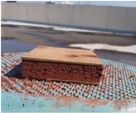
Fig 3. 12. Trimmed specimen for direct shear test
