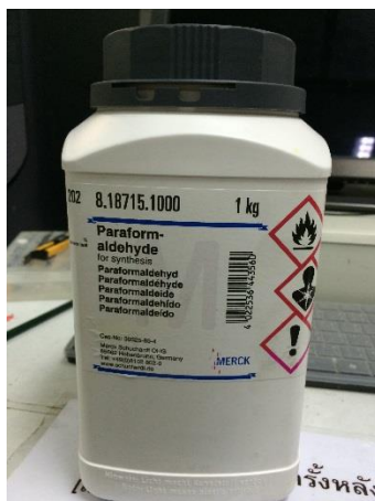
Figure 2.6 Paraformaldehyde powder used in benzoxazine synthesis.
