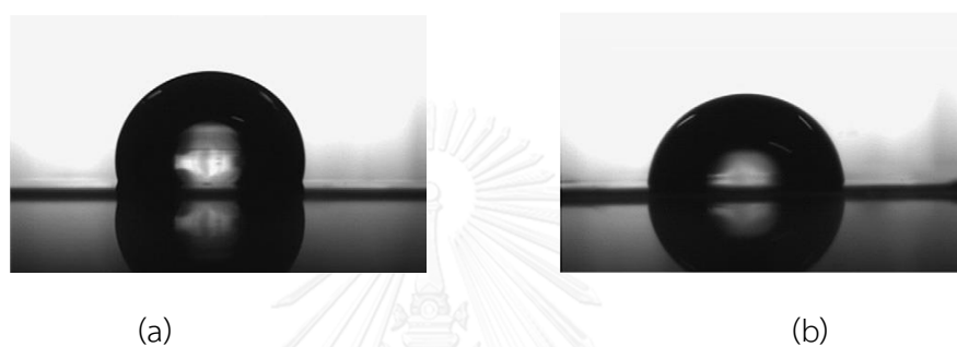
Figure 3.9 The profiles of a droplet water on the surface of polyimide film (a) fluorine-containing polyimide and (b) non-fluorine-containing polyimide.
