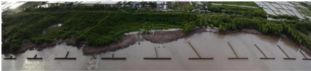
Figure 36 The model of T-shaped bamboo-fencing and its actual placement in the coastal zone of the lower Mekong Delta in Vietnam [33]
