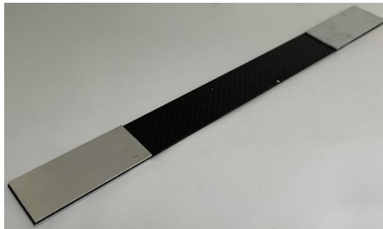
Figure 13 Carbon fibre reinforced polymer tensile test specimen.
