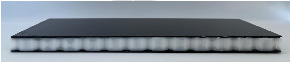
Figure 16 The sandwich composite beam with hexagonal core at relative density of
