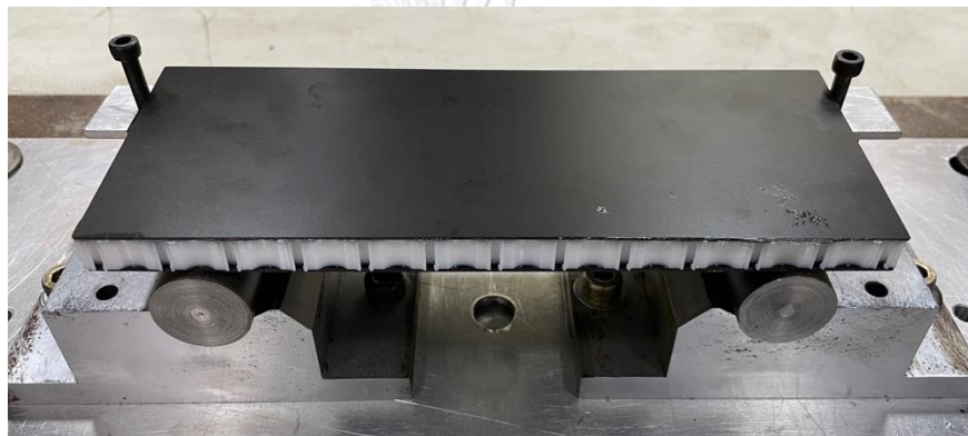
Figure 19 The specimen is fixed at the specify span length.
