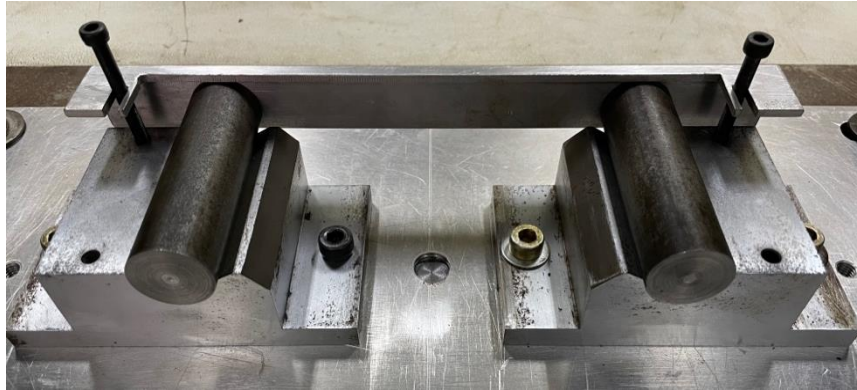
Figure 18 The partition device on three-point bending test.
