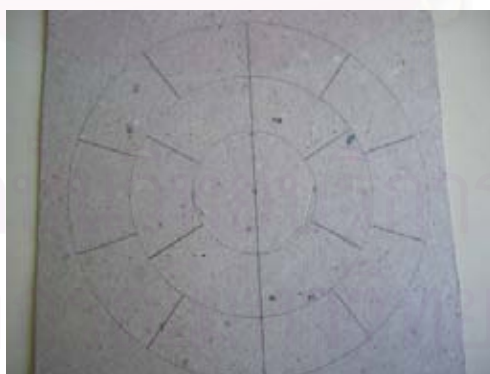
Figure 4.11 Paper Template for Determination of Film Thickness
