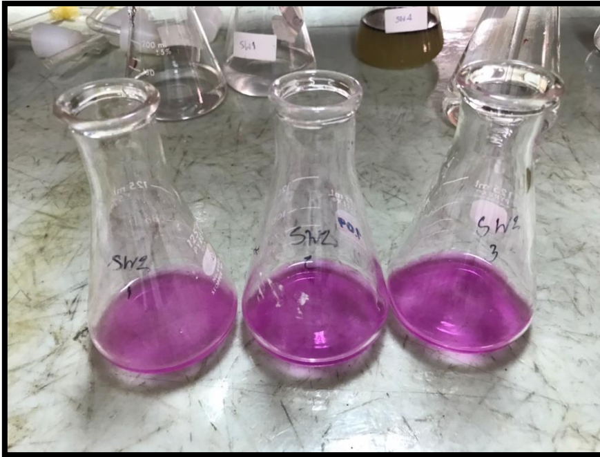
Figure 21 The color of the solution change to pink known as “End Point”.
