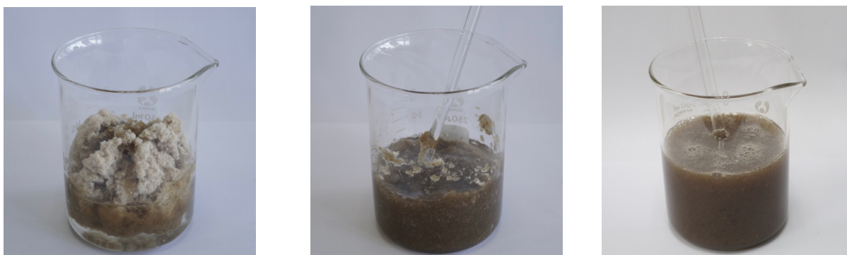
Figure 2-1 Acid hydrolysis of cellulose
