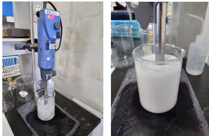
Figure 2-2 Regeneration of \text{BiPO}_4/\text{AC} from \text{Bi}(\text{NO}_3)_3 solution and amorphous cellulose from used envelop paper.
