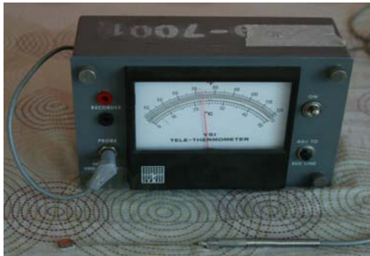
Fig 3.2 YSI tele – thermometer (Yellow Springs Instrument Co., Inc, Ohio, USA) with a factory calibrated thermister surface probe
