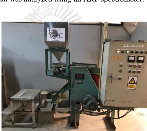
Fig. 4.1 Induced roll magnetic separator (ERIEZ MAGNETS CP887412 model, USA)
