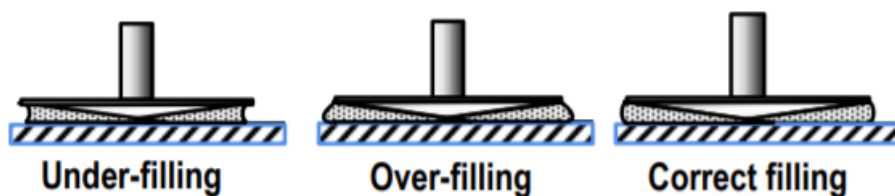
Figure 18 Proper loading of sample after closing the gap for cone and parallel plate geometry systems [61]
