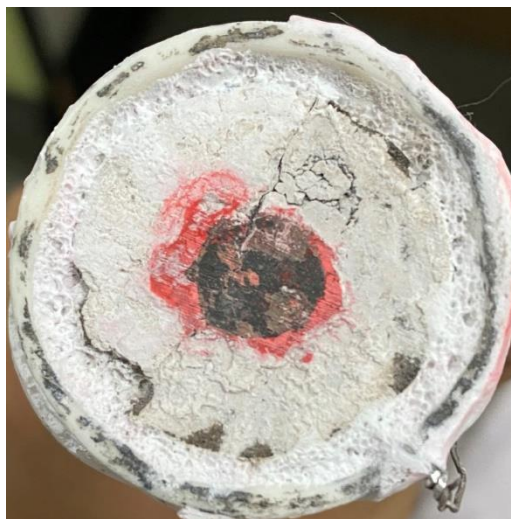
Figure 57 Image of Ni-Fe-alloy-foam supported SOEC after durability test operated at 0.9 and 0.3 \text{Acm}^{-2} with \text{H}_2\text{O}:\text{H}_2 = 70:30 at 1073 K, 10 h
