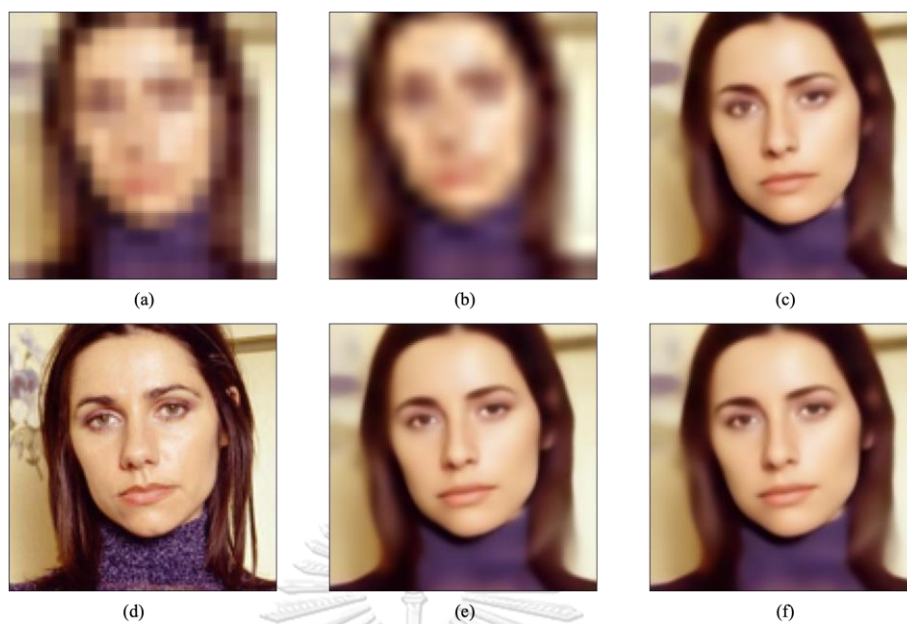
Figure 47. The comparison of face image in CelebA from 16x16 pixels to 128x128 pixels (7)
