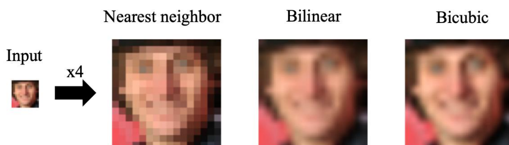
Figure 4. The comparison interpolation method of nearest neighbor, bilinear interpolation, and bicubic with scale x4.
